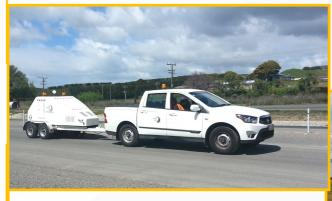
Pavement structural testing is required to ascertain pavement strength, and therefore performance. Data Collection Limited performs such pavement structural testing utilising JILS Falling Weight Deflectometer (FWD) and Heavy Weight Deflectometer (HWD).
